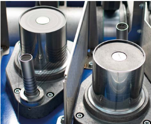
Fig. 4: Heated godets of TG30-PES
