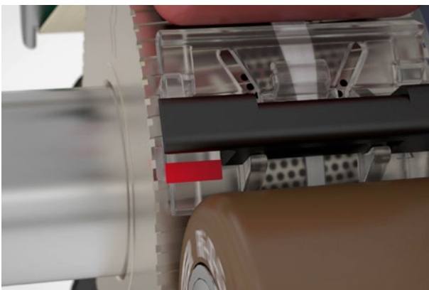
The red marking on the air guide element indicates that the compacting unit must be checked.
