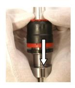
3) Press CROCOdoff in the direction of arrow at the picture. Use gentle force to overcome safety ring that keeps CROCOdoff in the correct position. 按照图中箭头所示方向压CROCOdoff。稍稍用力压过CROCOdoff卡圈,CROCOdoff会被卡圈固定在正确的位置。
