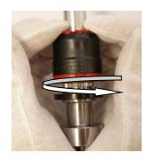
2) Find the right position of CROCOdoff by turning the part while applying a low force. The teeth of CROCOdoff must match the teeth of the wharve 稍稍用力转动CROCOdoff找到它的正确位置。CROCOdoff的齿必须与锭盘的齿相吻合。
