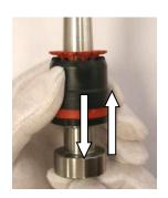
4) Check the correct function of CROCOdoff by opening and closing it. Both movements must be smooth.
