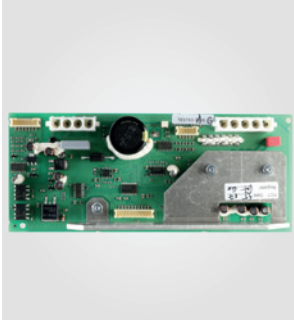
Winding head drive unit 171-670.033
