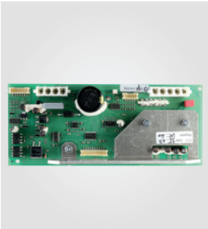
Winding head drive unit 171-670.033
