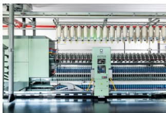
Fig. 1: With the fully electronic ring spinning machine G 38 equipped with the piecing robot ROBOspin, Beste Spa produces yarns of highest quality.
