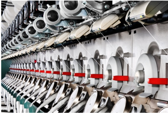
Image caption: The CHANNELpass optimises yarn strength and the number of neps with rotor spinning.
