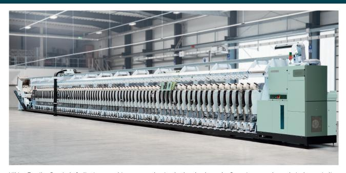
Viking Textiles Pvt. Ltd., India, increased its yarn production by 1% thanks to the Smartjet upgrade on their three winding machines Autoconer 6. The Smartjet power nozzle helps to increase the efficiency of the suction nozzle's upper yarn search and pick-up from the package. This reduces the operator's workload in attending the packages during red light stoppages of the winding units.
