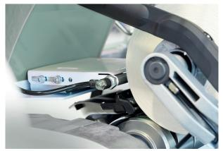
The Smartjet upgrade installed in the doffer unit helps improve the efficiency of the upper yarn search.
