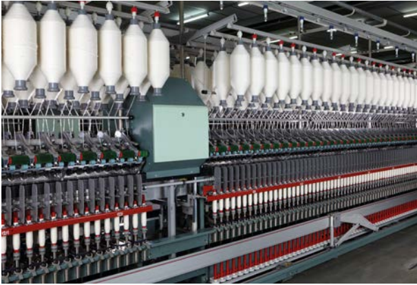
Ring spinning machine G 32 – for the production of high-quality yarns produced with high efficiency
