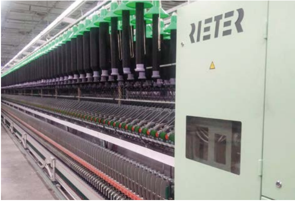
Ring Spinning Machine G 32 – a top quality machine that combines efficient energy utilization and superior yarn quality with high spinning speeds
