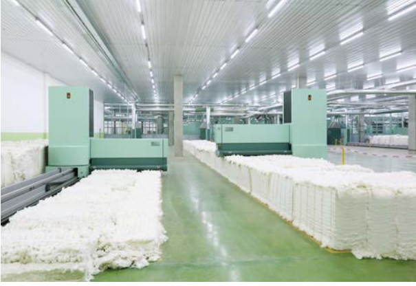
Six UNIfloc A 12 bale openers supply the compact spinning machine K 46
