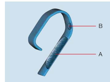
Ring traveler weight too light Excessive wear in area A
