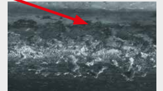
Worn-out steel ring
