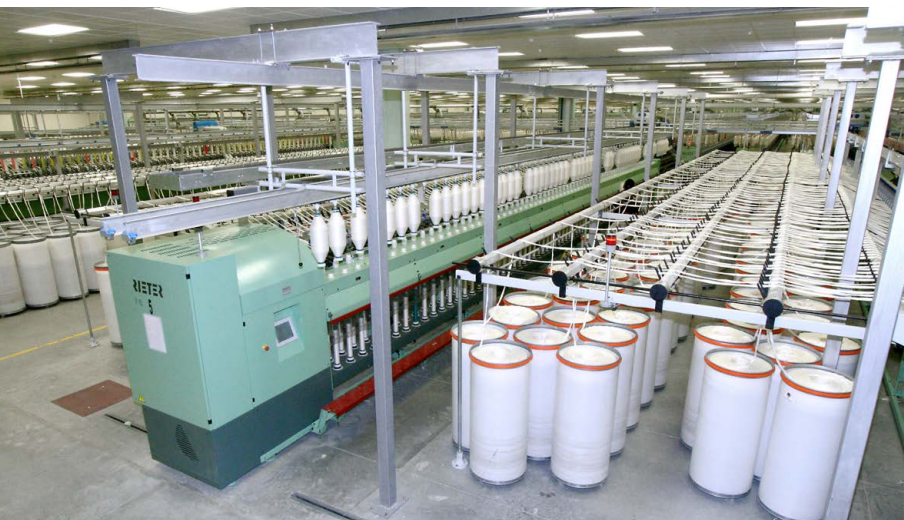
Fig. 2 Irrespective of the can content, the plates with the raw material are always straight and at practically the same height, which ensures the sliver quality.
