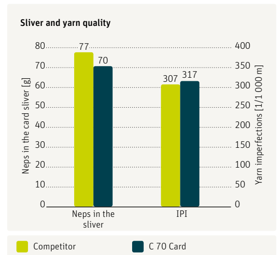
Fig. 2 With clearly higher production, the Rieter line achieves equally good sliver and yarn quality.
