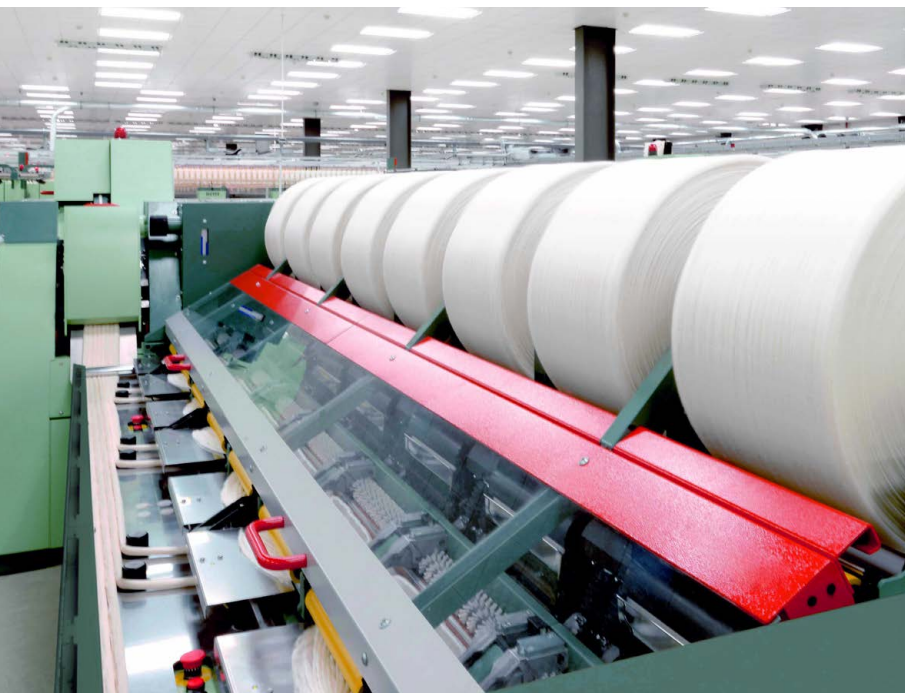
Fig. 5 The E 86 with higher cleaning level: fewer trash particles without fibre damage.
