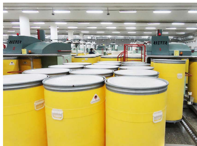
Fig.3 Handles on the cans ensure good sliver quality – the sliver in the can stays untouched.
