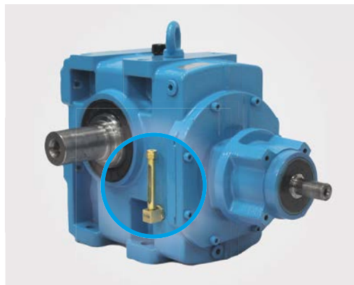
Repaired gearbox with oil indicator for 3.0 L
